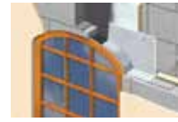
Parabolic Arch lintel
